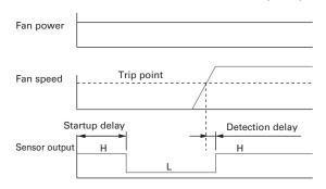
Startup delay: 18±3 sec. Detection delay: 3 sec. MAX. Trip point: 1700 min-1
